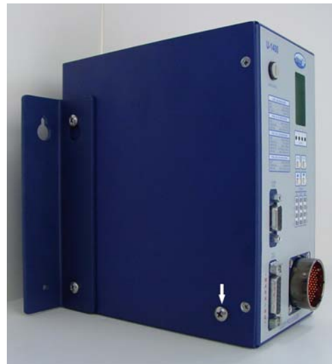
Unused Hole - Wall Mount (Left Side Shown, Right Side Similar)
