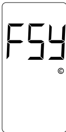
Parallel Synch Mode Failure Indication
