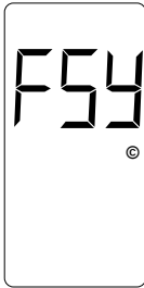
Series Synch Mode Failure Indication
