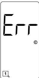
**Detection Reference Error.** This is an indication that the internal EEPROM and the motherboard mounted EEPROM detection reference values do not match. Press the FUNC button to clear the error message.
