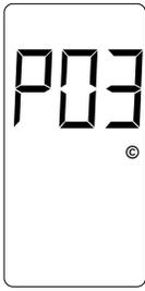
Upon application of power, the LCD screen will show the detector model letter and firmware version, in this case, Model P-1400 firmware version 3. This screen will be displayed for two seconds.
