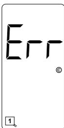
**Detection Reference Error.** This is an indication that the internal EEPROM and the external EEPROM memory module detection reference values do not match. Press the FUNC button to clear the error message.
