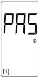
The detector will next confirm the state of the check loops connected to it. If all four check loops are connected and are intact, the LCD screen will display an indication of the successful completion of the check loop verification. This screen will flash twice.
