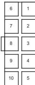
Slot 0 - J40 (Optional) Slot 1 - J42 Slot 2 - J43 Slot 3 - J44 Slot 4 - J45 Slot 5 - J46 Slot 6 - J47 Slot 7 - J48 Slot 8 - J49
