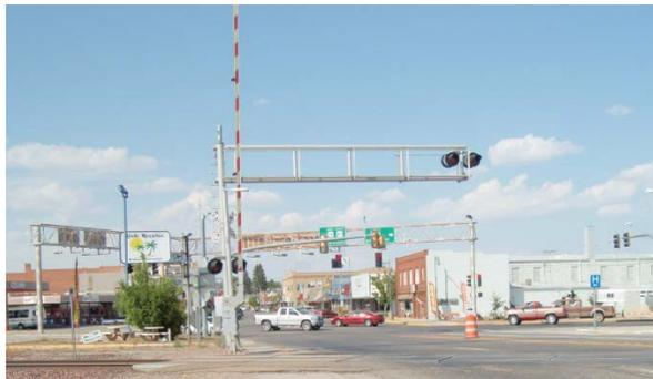
*The grade crossing at U.S. 85 and Main Street in Torrington, Wyo., will be one of the first locations in the state in which a wayside horn system will be installed.*
